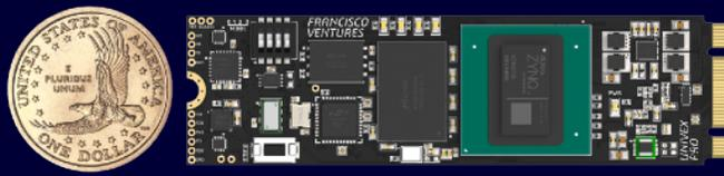
The embeddable UNIVEX™ Pro & QUAM™ Q7 series integrates a powerful Xilinx® MPSOC Ultrascale+ core for secure, high performance design flexibility and unique protection, combining physical sensors with top-notch security elements. These rich features create a complete, isolated and secure embedded computer in a tiny Mini-PCIe or M.2 form factor.
